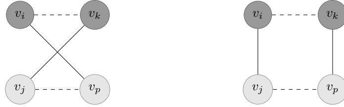
Figure 8.5: Valid switch operation among vertices v_i, v_j, v_k and v_p (dashed lines represent deleted edges while solid lines are the added ones).
